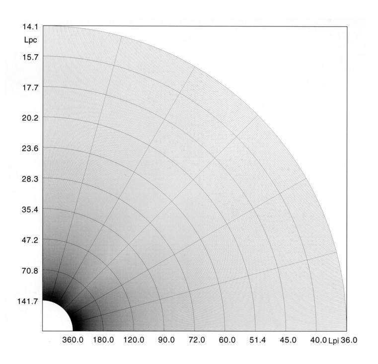
The Zero Line Width graphic was toner printed by 1200x1200dpi/121Lpi/45°. The print was scanned with 1200dpi,blurred and downsampled for 144dpi (optimal for PDF zoom 200% at 72 dpi resolution).
