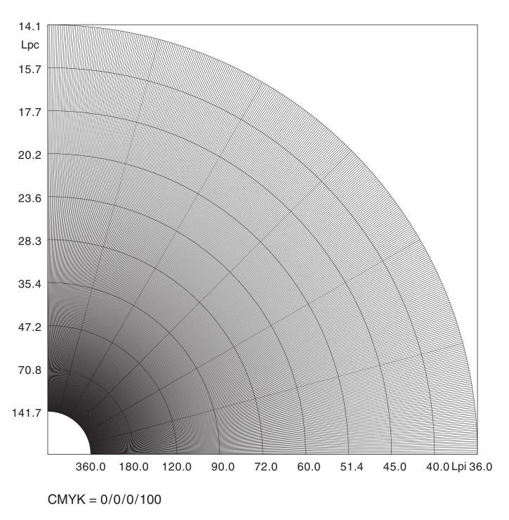
The radial lines are programmed with zero line width. PostScript interpreters assign the smallest printable width, but this is not well defined.
