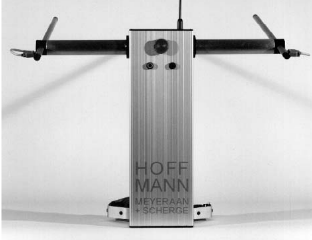
Fig.2 Motography Rucksack, four LEDs on a square
